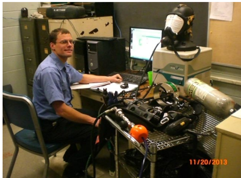
Lt. Andrew Finson conducting the annual in-house servicing of the SCBA (Self-Contained Breathing Apparatus) equipment. The servicing includes testing of the air regulators and air packs.
